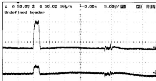
Figure 5: Compensation of the beam loading at injection with the feed-forward. I/Q components of  $V_t$  (AC coupled): The time window ( $5\mu s$  per div.) shows the first turn where no compensation can be applied, and the second turn (after one revolution period  $T_{rev} = 23\mu s$ ) with the full correction from the feed-forward. (One batch of 72 bunches,  $0.7 \times 10^{11}$  protons per bunch, four sections cavity, MD session 2<sup>nd</sup> Nov. 2000).
