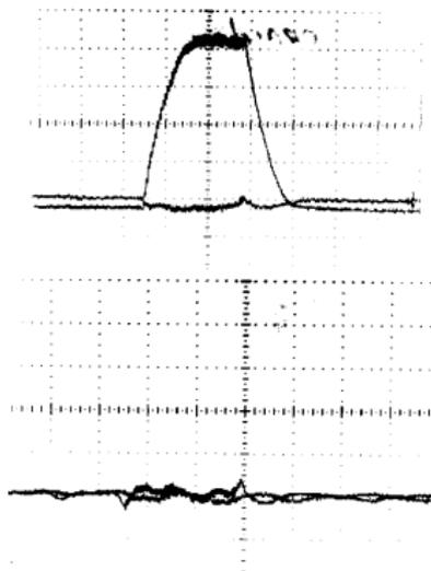
Figure 16: I/Q components of  $V_i$  (AC coupled) 1 ms after injection (500 ns per div.). Top: no compensation. Bottom: feed-forward and feedback pair on. Beam conditions as in Figure 11.
