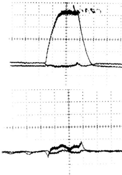
Figure 12: I/Q components of  $V_i$  (AC coupled) 1 ms after injection (500 ns per div.). Top: no compensation feed-back on. Beam conditions as in Figure 11.
