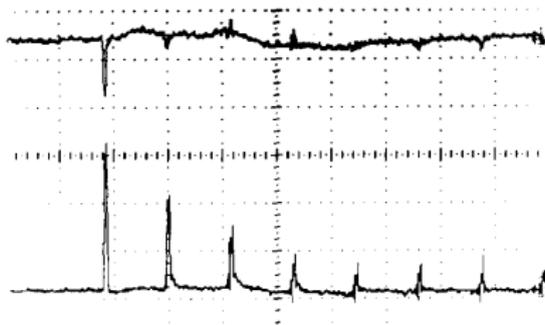
Figure 11: Compensation of the beam loading at injection with the feed-back. I/Q components of  $V_t$  (AC coupled) showing the progressive compensation turn after turn,  $20\mu s$  per div.,  $T_{rev} = 23\mu s$ . (One batch of 48 bunches,  $0.83 \times 10^{11}$  protons per bunch, four sections cavity, MD session 30<sup>th</sup> Aug. 2000).
