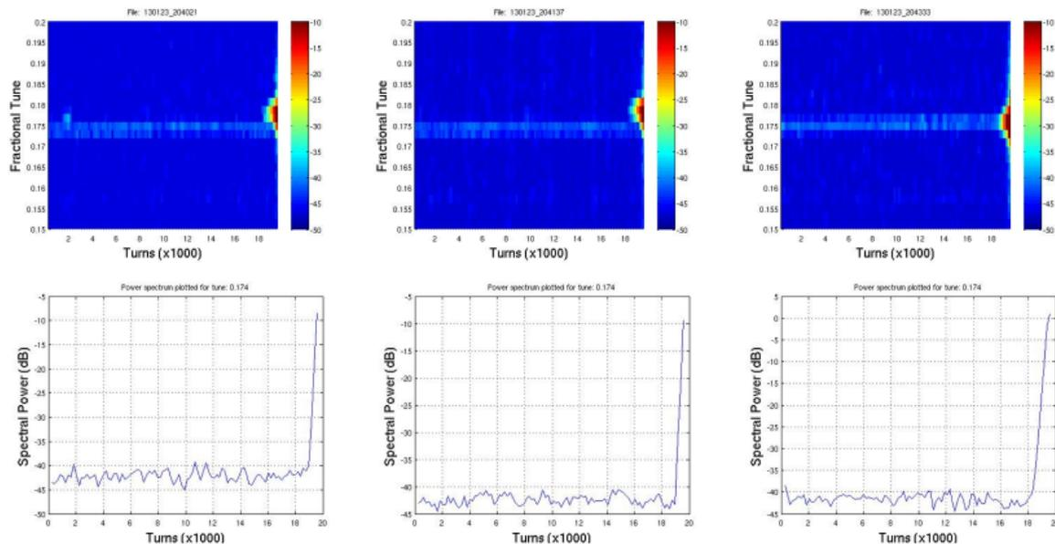
Feedback is switched off at turn 18K, beam then is unstable
