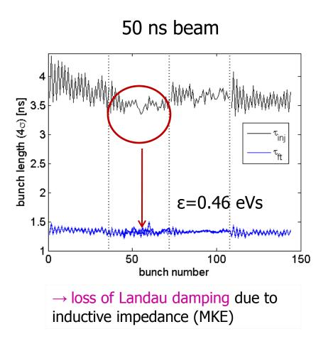
Narrow window for the injected parameters: losses increase for longer bunches and beam is unstable for lower emittance (blow-up required for 50&75 ns beams)
