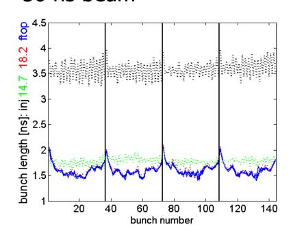
Non-uniform emittance blow-up due to beam loading in a double RF system
