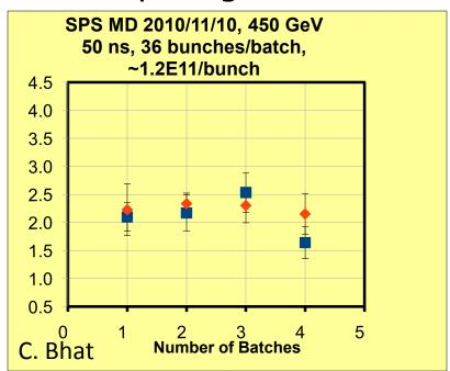
No emittance increase with n batches, small (<10%) blow-up during the cycle
