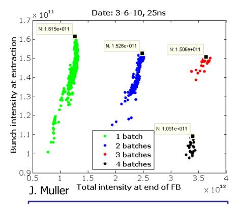
Bunch intensity on flat top decreases with number of batches:  $1.62 \times 10^{11}$  -1 batch,  $1.51 \times 10^{11}$  - 3 Beam losses:  $30\% \rightarrow 20\%$
