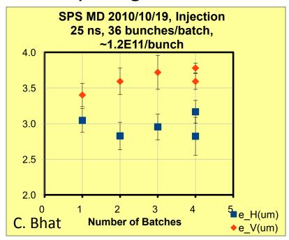
Vertical emittance increase with n batches, measurement at 0.55 s (26 GeV)
