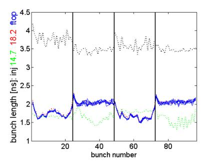
Non-uniform emittance blow-up and beam instability (?) for short injected bunches
