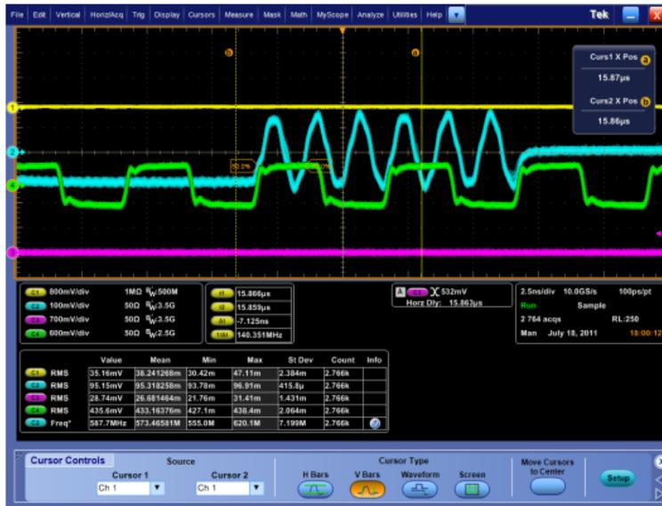
Injection trigger- (magenta), Rev-Markers (yellow), Excitation signal (light blue ), 200MHz reference signal (SPS ring - green)
