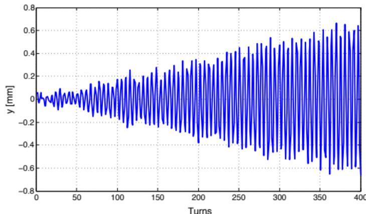
Kicker signal for all the slices:  $V_b = 4.10^{-6} \sin(2\pi 0.185 \text{ Turns})$  eV.s/m. C-MAD result: Vertical displacement of center of the bunch.
