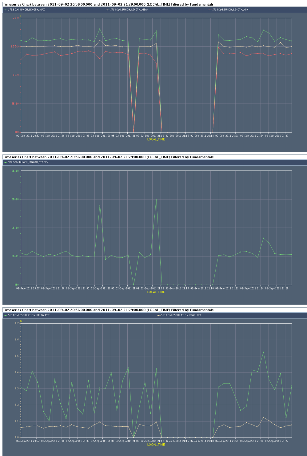
Figure 7: 72 bunches, 25 ns beam, Q20 optics. Top: BQM variables BUNCH_LENGTH_MAX, BUNCH_LENGTH_MEAN and BUNCH_LENGTH_MIN. Centre: BUNCH_LENGTH_STD. Bottom: OSCILLATION_DELTA_PCT and OSCILLATION_PEAK_PCT. At 21:05H there had been a bad cycle, the cycle at 21:12H occurred just before the beam was cut by the CPS at 21:13H due to an RF intervention was also a bad cycle. Data acquired between 20:56H to 21:29H, 2011-09-02.
