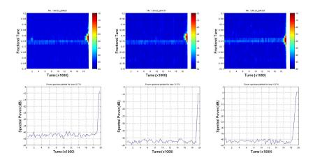
Feedback is switched off at turn 18K, beam then is unstable
